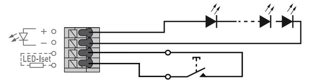
Helvar Components' innovative Direct Control (patent pending) behaves much like the Switch-Control, but in this case the control can be implemented in a more straightforward way without using the mains voltage. Only a simple retractive (push to make) switch connected into the Iset / LED-Iset terminal and enabling the Direct Control from the Helvar Driver Configurator tool are needed. DALI usage is **not supported** at the same time with Direct Control operation.
