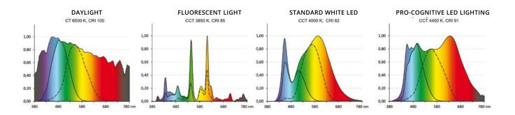
Comparison of spectral composition and biological (full curve) and visual (dashed curve) efficiency of daylight, fluorescent light, standard white LED and bio-optimised pro-cognitive LED lighting, source: Lenka Maierová, ČVUT UCEEB
